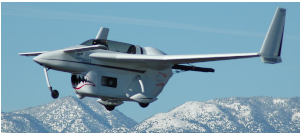
Figure 5 The first PDE-powered aircraft flies over a Mojave desert in 2008 [63].
