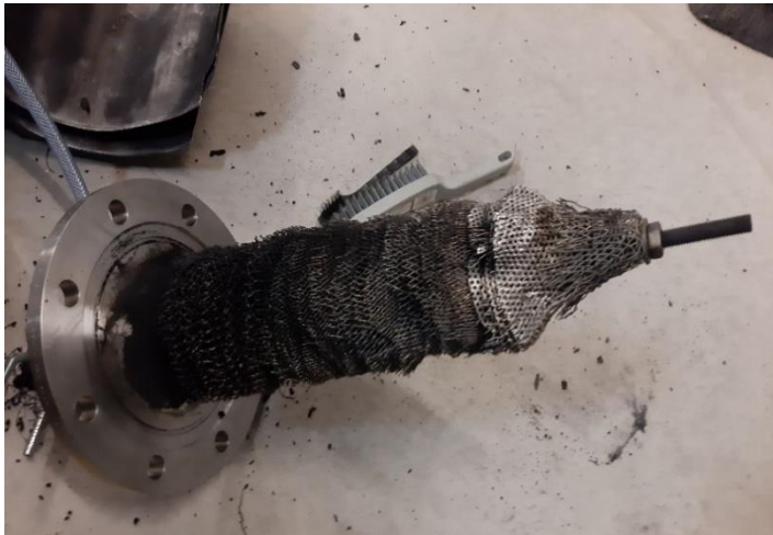
Figure 19 The inside of the dumping section: a) the damaged mesh circles after a number of experiments; b) new portion of the mesh circles added on the top of the old ones.
