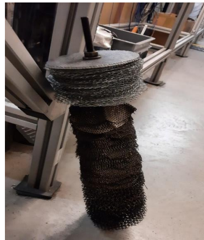
Figure 19 The inside of the dumping section: a) the damaged mesh circles after a number of experiments; b) new portion of the mesh circles added on the top of the old ones.
